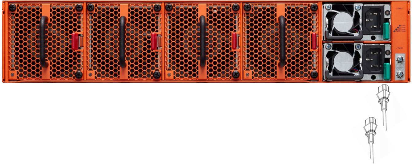
Figure 4-5: Connecting AC Power on a GigaVUE-TA200
